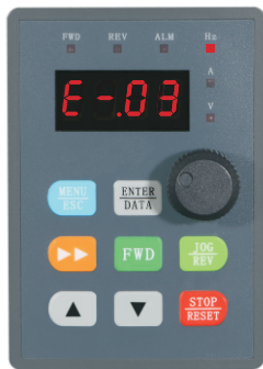
Figure 4-5 Fault alarm display state
